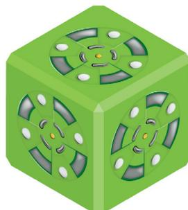
The dark green Blocker Cubelet differs from the bright green Passive Cubelet. The Blocker Cubelet does NOT pass data but allows power to flow. The Passive Cubelet passes BOTH power and data.
