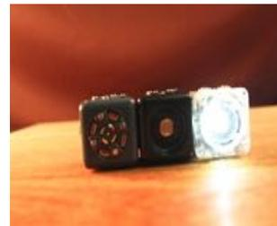
“Robots are automatic agents that can sense, think, and act. Our robot senses are in these black cubes. Our robot action parts are in these clear cubes. Also, all robots need power, and the gray blocks are the battery or power cubes. We’ll use the Brightness sense first and the Flashlight to see how input and output work together“
